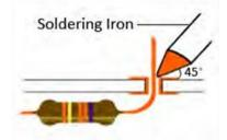
Step 7: Touch the solder to the iron tip and move that around the joint by keeping the iron tip fixed. Let the solder melt and flow till the joint is covered, as shown in the following figure:
