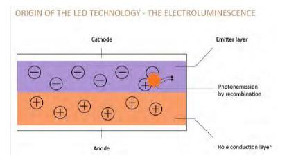
In LED chips, on application of certain voltage, electromagnetic radiation in the form of light is given out.
