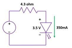
Indicator LEDs are generally powered by this method. For lighting applications, there are some drawbacks of this method and one of them is inefficiency. There is loss of power across the resistor in the form of heat. For example, if a 10V source is used to provide power
