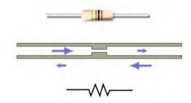
Resistance is measured in Ohms ( $\Omega$ ) 1000 $\Omega$  = 1k $\Omega$ , 1,000,000 $\Omega$  = 1M $\Omega$
