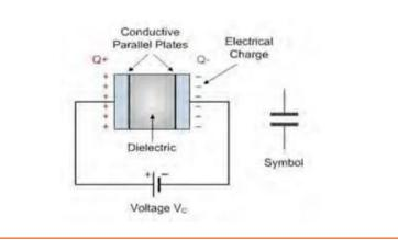
The plates store the energy of the electrons as electrical charge on, which means, greater the plates and lesser the distance, more will be the capacitance.
