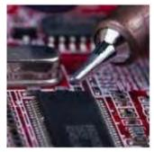
The tip can be changed by an easy process that involves either unscrewing the wand or applying pressure inwards and pulling out the tip.
